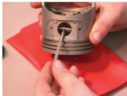
Figure 57-50. Measure the piston pin in the locations shown to determine wear.
